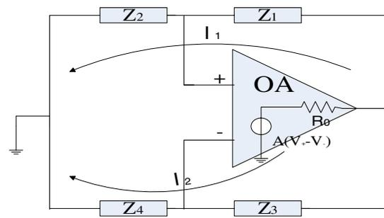
Fig. 3 Generalized Wien bridge oscillator
