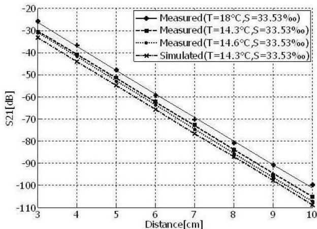
Fig. 7. Sea water transmission ( $S_{21dB}$ ) at nominal frequency vs separation distance for different measurements series compared to EM simulation.
