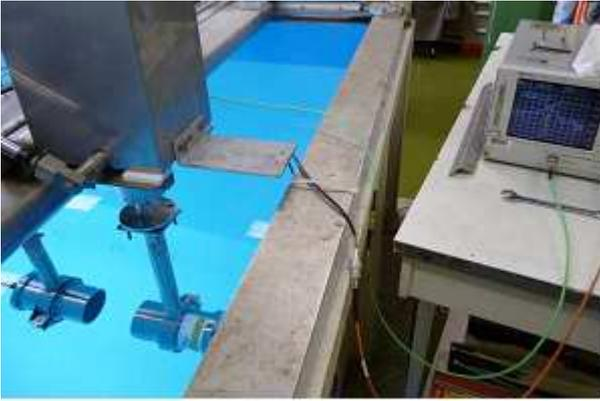
Fig. 2. Transmission measurement between the antennas in freshwater basin
