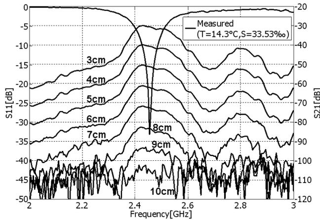
Fig. 6. Reflection ( $S_{11dB}$ ) and transmission ( $S_{21dB}$ ) sea water measurements for several antennas separation distances
