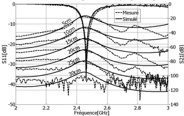
Fig. 3. S11 et S21 measurements compared to EM simulations
