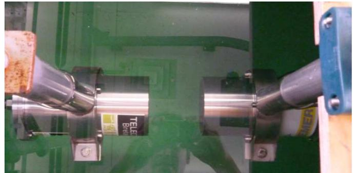
Fig. 5. The two antennas immersed in the basin filled with sea water
