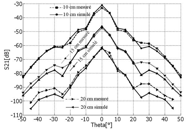
Fig. 4. Transmission depending on azimuth angular position of the antennas, for 10, 15 and 20 cm separation distances
